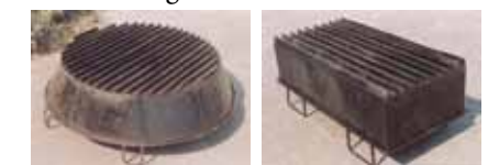
Fig. 2. Modified main and gutter pans of IISR 2-pan furnace
