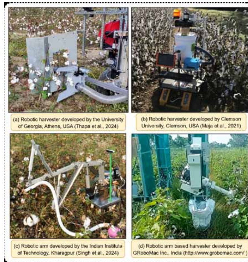
Figure 2: Example of ongoing research effort on robotic harvester in USA and India.
