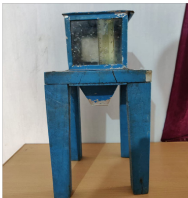
Fig. 1. Angle of repose measuring setup.
