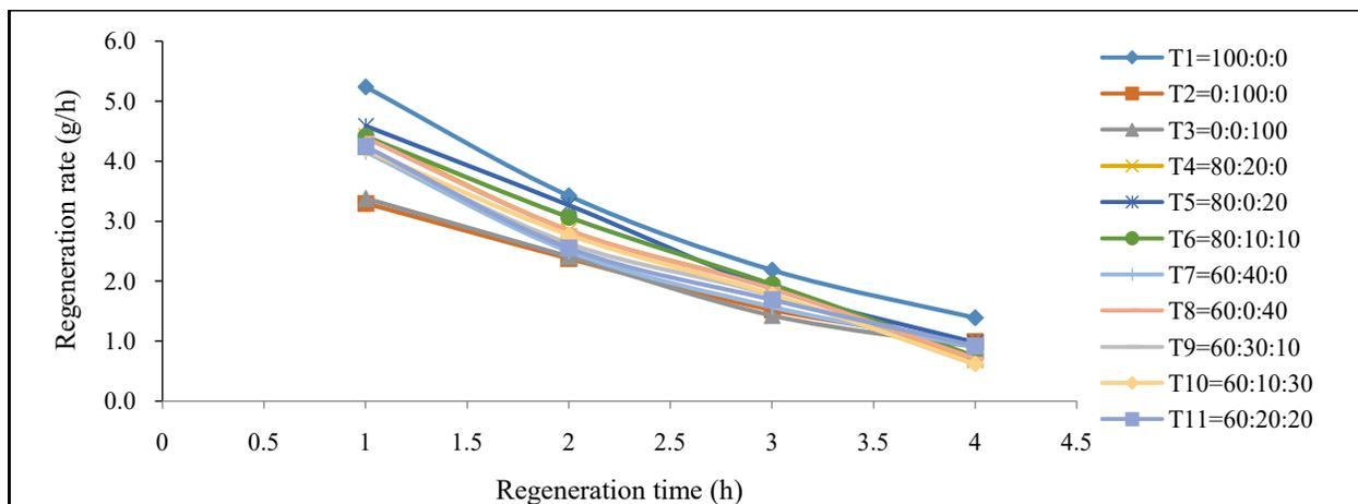
**Fig. 3.** Regeneration rate of different composite desiccants at 55°C
