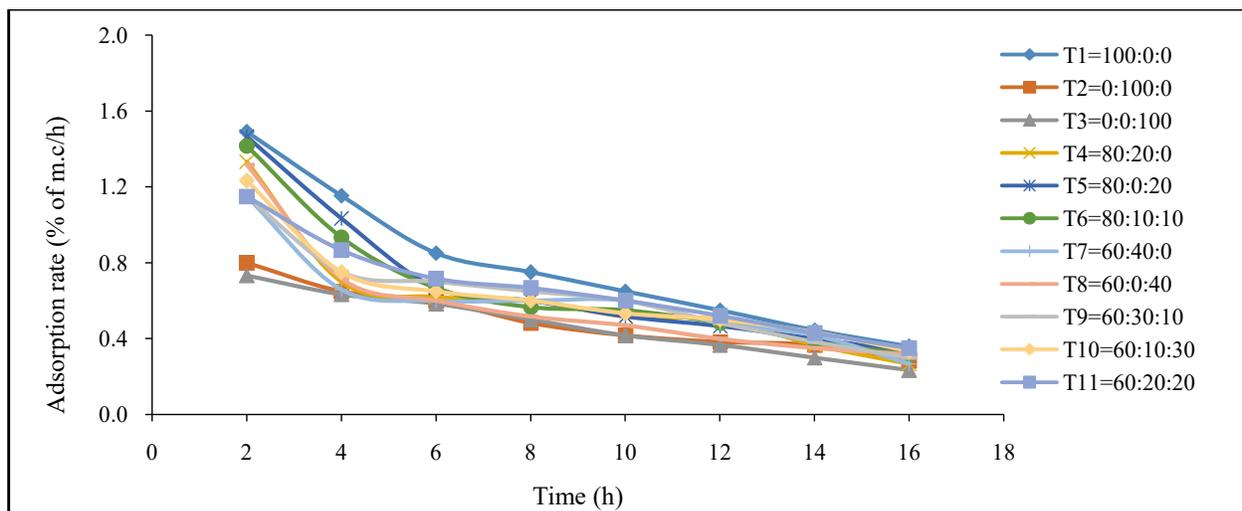
Fig. 2. Adsorption characteristics of different composite desiccants
