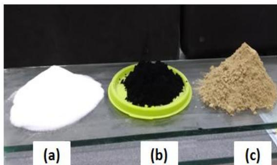
**Fig. 1.** Selected desiccants (a-silica gel; b-activated carbon; c-bentonite clay) for preparation of composite desiccant
