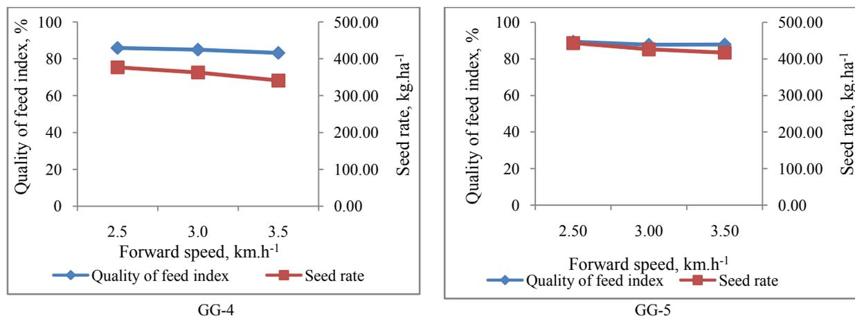
**Fig. 7: Effect of forward speed on quality of feed index and seed rate of garlic clove during field test of tractor operated garlic clove planter**
