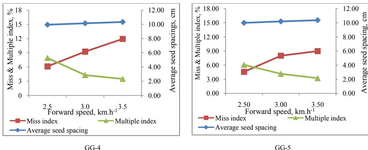
**Fig. 6: Effect of forward speed on average seed spacing, miss index, and multiple index of garlic clove during field test of tractor operated garlic clove planter**
