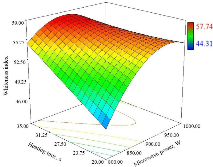
**Fig. 3: Effect of microwave power and heating time on whiteness index of puffed brown rice**
