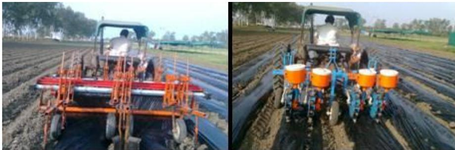
A plastic mulch laying machine for positive release of film was developed to lay the plastic film on broad beds and have the soil edges of the film buried in soil from both sides. The unit was tested for planting French bean at CIAE, Bhopal
